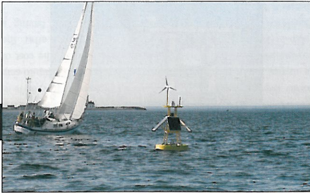
The Littoral Sensor Grid buoys transmit video and environmental data over a floating area network.
